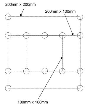
**Figure 1.** Typical VESA Mounting Hole configurations
